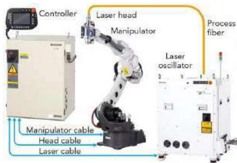
Figure 3. The main components and connection of the Laser Processing Robot Integrated System Solution (LAPRISS).
