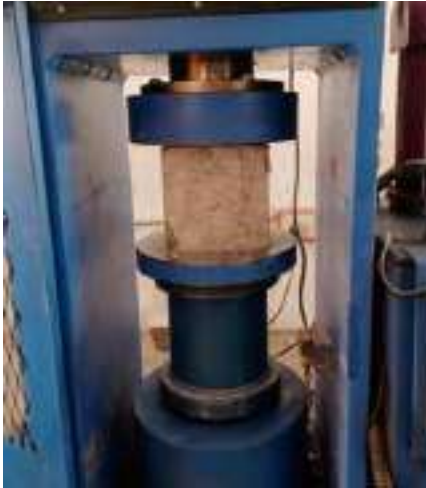
Figure 1. Compressive strength test setup
