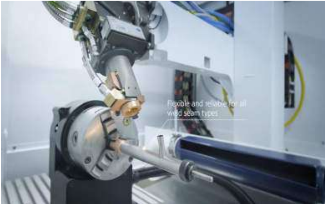
Figure 4. Automated Laser Welding ( fractory.com/laser-welding. , 2024) (Trumpf Laser Welding TruLaser Station 7000).
